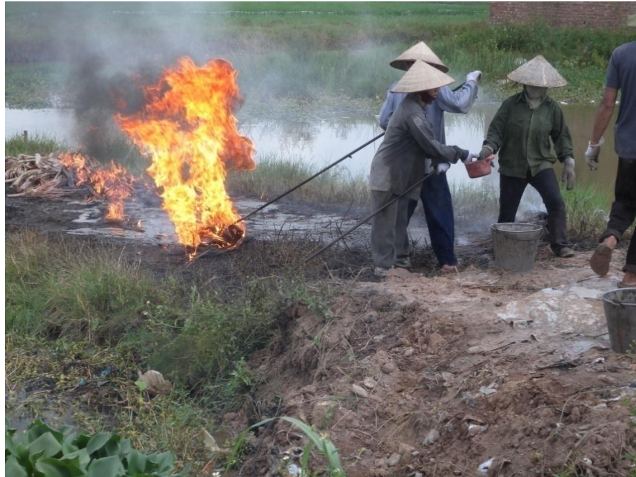
Open burning of plastic-coated wire to extract copper. Vietnam, August 2009.
