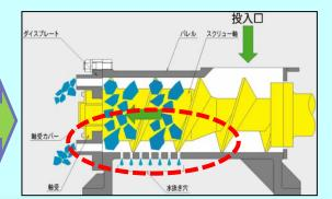
Water discharge function for high calorific value
